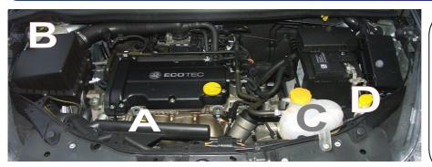
A = Dipstick B= Brake Fluid Reservoir C= Coolant D= Washer Reservoir
